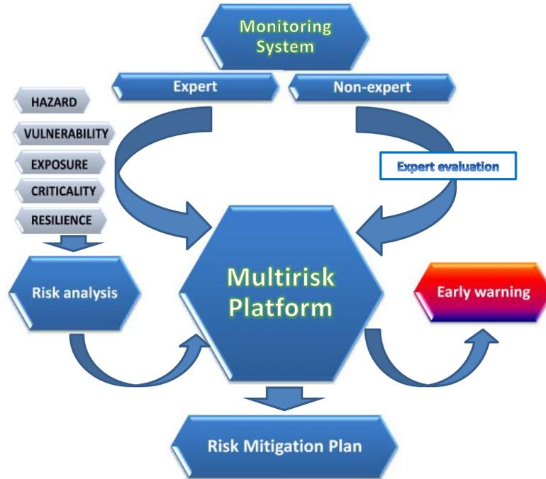
Figure 3 clarifies the role played by the Multirisk Platform that may be considered as the intelligent centre of the complete emergency management system, because it takes into account all the natural risks, constantly checking the component elements that compose them, arranging the update of the Mitigation Risk Plan and activate the Early Warning System.
